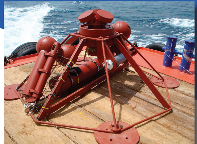
Example of acoustic Doppler profiler prepared with anti-fouling paint. This ADP was deployed in 83m of water near to the Iranian border in the Strait of Hormuz, Middle East. The equipment was raised every 3 months, swapped and redeployed lasting 18 months. Photo courtesy of Darren Birmingham, HDR Engineering.
